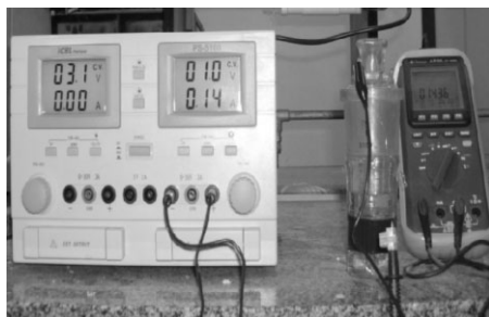
Figure 1. Overall view of the home-made apparatus for conductivity measurements.
